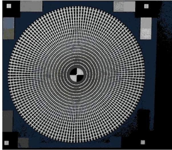
Figure 6: For 24 segments the border of the star is detected and results in a distortion corrected analysis.
