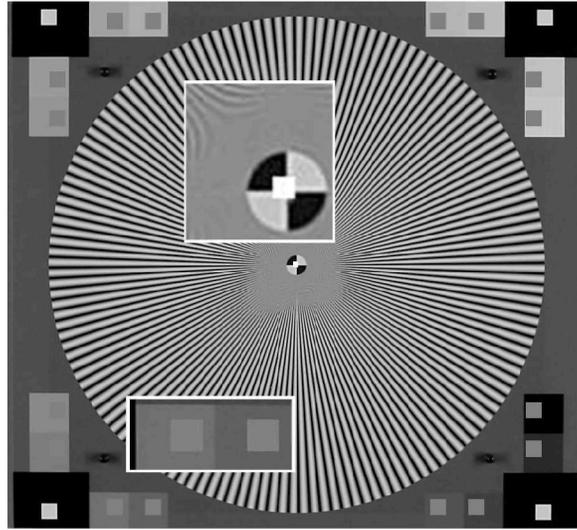
Figure 5. Chosen positions of the OECF patches and the center of the star number 0
