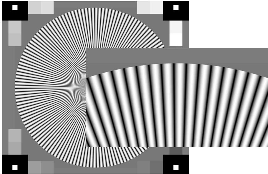
Figure 2: A sinusoidal Siemens Star appeared to be the ideal structure to test the resolution of cameras. The Star is surrounded by 16 Grey patches, which are used to linearize the image prior to the analysis. A central marc helps to get the focus right and to fine tune the detection of the center.
