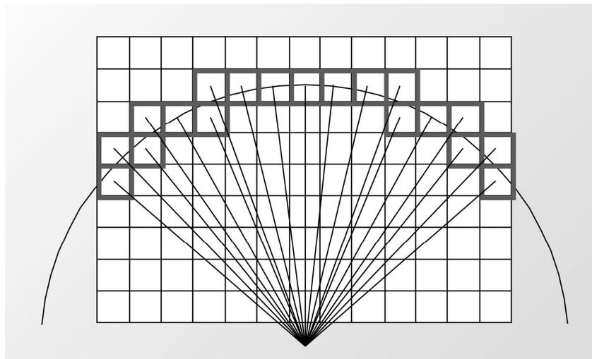
Figure 7: Chosen pixels along a circle of a siemens star
