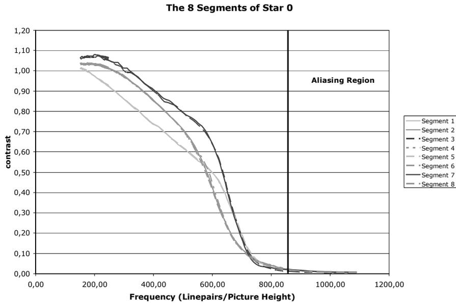
The shape of the SFRs for the segments of the center star shown in figure 10 appears to be different. This indicates either an orientation specific image processing or a special sensor geometry that prefers a specific orientation.
