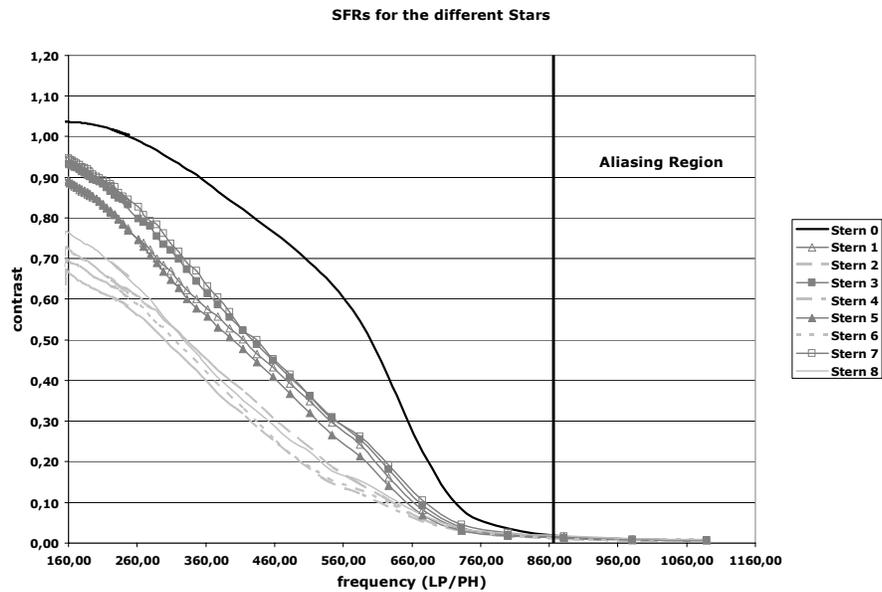
Figure 11: SFRs for the nine stars in the image taken with a camera that has a well centered lens
