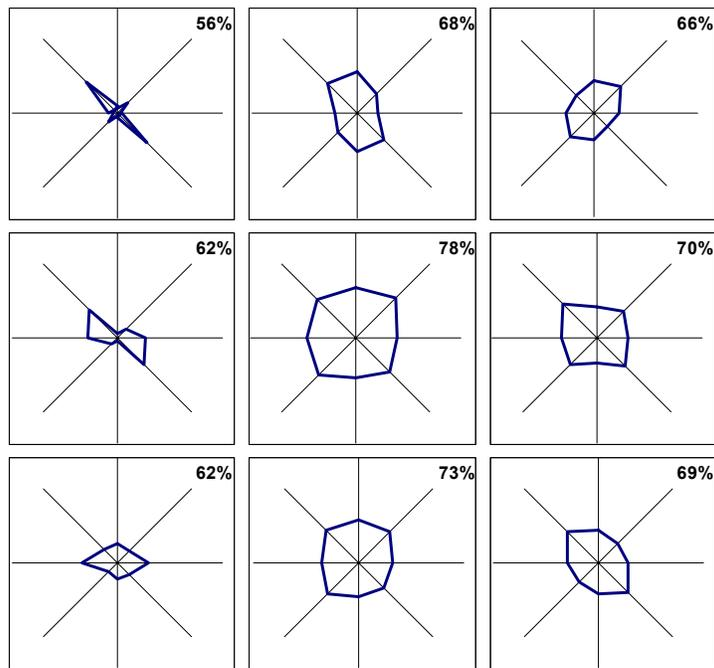
Figure 16: The limiting resolution for the 8 Segments of all 9 stars. The values are given in percent of Nyquist.
