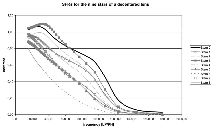
Figure 12: SFRs of a camera with a decentered lens
