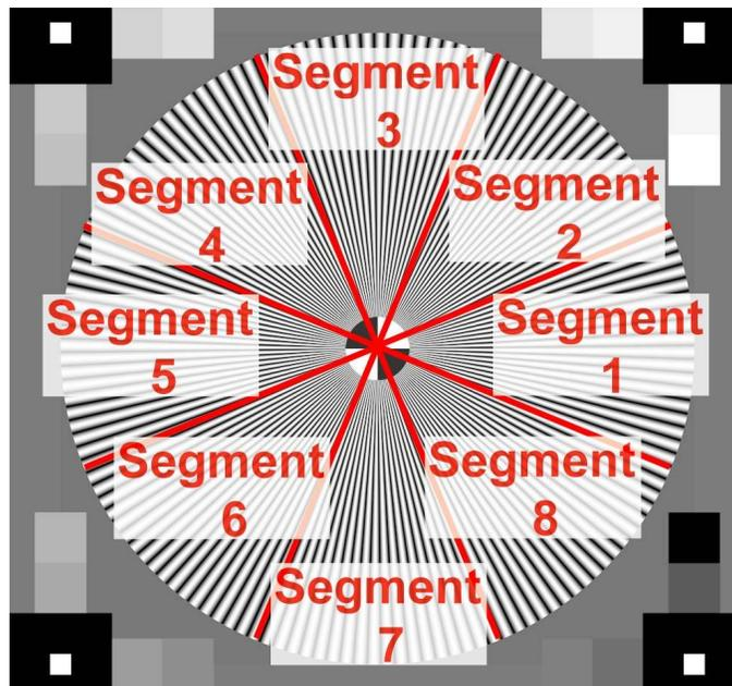
Figure 4: For the evaluation each Star is divided into 8 Segments numbered as marked above.
