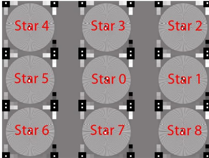
Figure 3: The standard target consists of nine sinusoidal Siemens Stars aligned in three columns and numbered as shown here.
