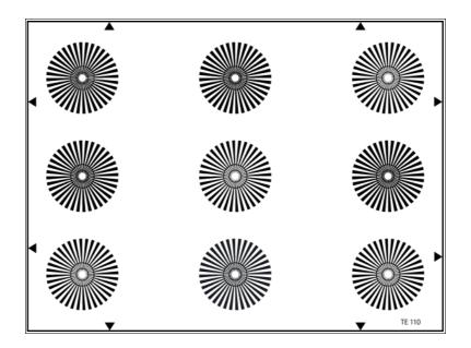
The test chart consists of 9 sector stars, distributed equally over the picture area. The unresolved center of the sector star is 10% of its outer diameter. Within the sector stars are two circular lines. The inner one marks a 625 line structure, the larger circular line marks a structure of 312 lines.
