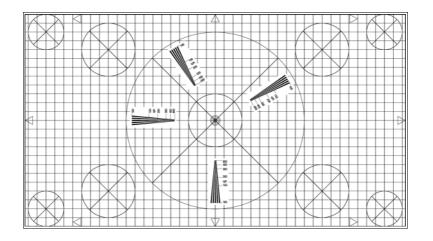
A grid structure consisting of 23 horizontal and 43 vertical lines is arranged on a white background forming 24x42 squares. The width of the grid lines is 0.08% of the picture width. The large circular line has a diameter of 83 1/3% of the picture height, the 5 small circular lines in the 4:3 area have a diameter of 25% of the picture height, the 5 small circular lines in the 16:9 area have a diameter of 16 2/3 % of the picture height.
