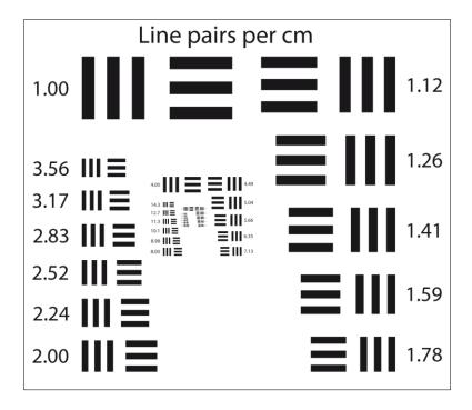
This chart is designed for resolution measurements.
