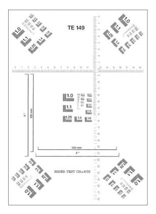
The test chart can be supplied as a foil or a reflectance chart, alternatively positive (see fig.) or negative. The foil is available on 0.10 or 0.18 mm thickness. Image end external size is 297 x 210 mm (DIN A4).
