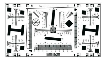
The TE170 is designed to measure resolution of still cameras.
