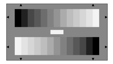
Two 13-graduated counter current gray scales are arranged on a gray background (D = 0.75), the gray scales being graduated logarithmically. Related to the densities of the gray scales: gamma = 0.45, related to the transmission values (brightness): gamma = 2.2, that being exactly the reciprocal value of gamma = 0.45. The output signal of a optimally gamma-corrected camera yields two 13-graduated counter current linear step signals.
