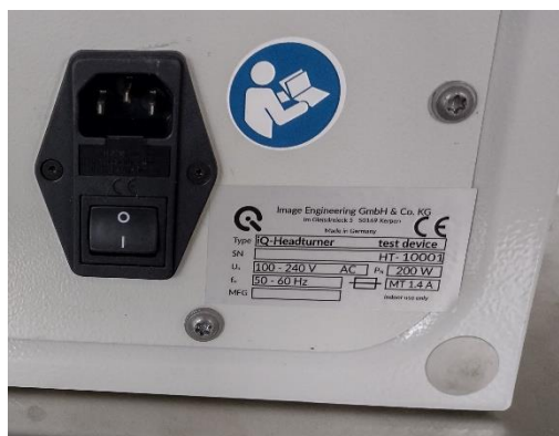
Figure 5 Main switch and nameplate
