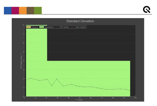
The tolerance range, that is defined in the specifications, is displayed in green. Values that are outside the tolerance range are outlined in red *"Value Violation"*.
