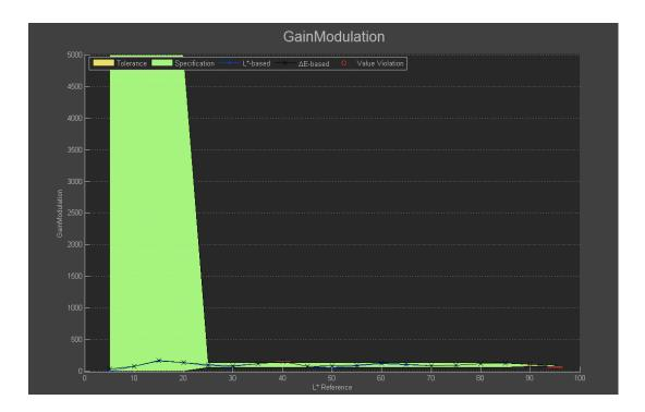
The thin black line represents the gain modulation based on  $\Delta E$ , the blue line represents the gain modulation based on  $L^*$ . The tolerance range, that is defined in the specifications, is displayed in green. Values that are outside the tolerance range are outlined in red *"Value Violation"*.
