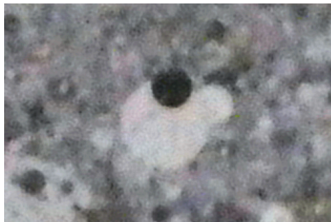
Figure 18. Example image Nikon S1000pj. enlarged (4x), dead leaves target at ISO1600. The image content is covered by noise introduced by the camera's internal processing. Results in Figure 17. The results would lead to the conclusion, that the dead leaves MTF or Gaussian power spectrum is better than for the other methods, which is wrong.
