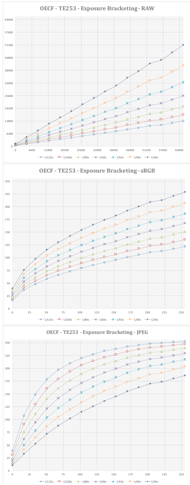
Figure 5. OECF (meanvalue of Y-Channel vs. idealized reflection, scaled to match image data range); measured based on linearization gray patches in a harmonic Siemens star (see Fig. 3); Constant ISO speed and f-stop, changing exposure time; top: Y_{linear} , extracted from camera RAW file; center: Y_{sRGB} standard sRGB Tone Curve applied; bottom: Y_{sRGB} based on JPEG output of camera
