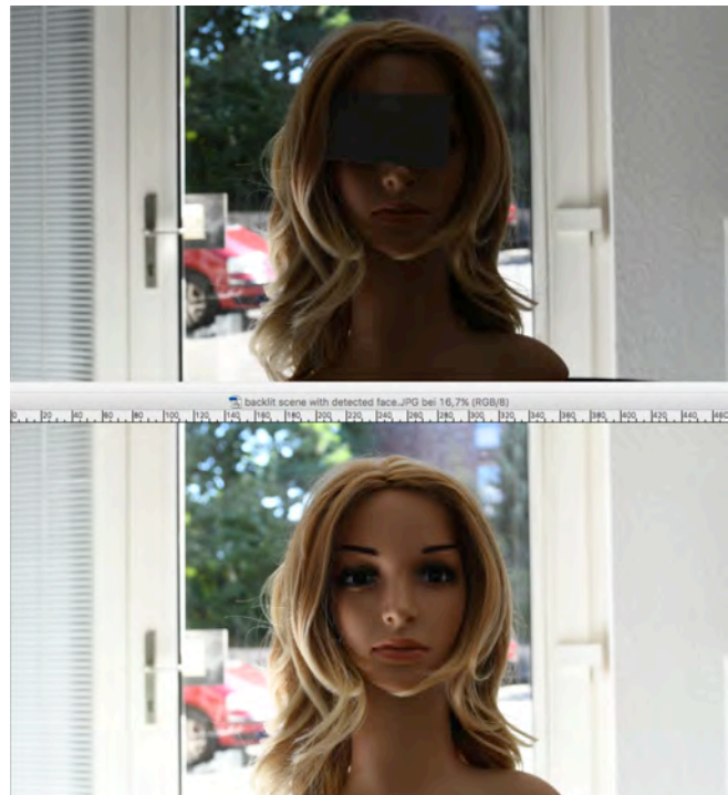
Figure 2: The impact of face detection on the exposure and image processing in a camera. In the upper image of this backlit scene the face is covered and in the lower image the face was detected.
