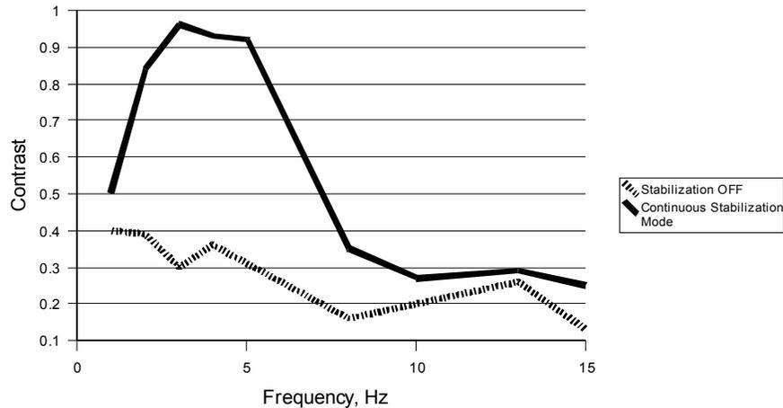
**Figure 9.** Contrast values at 300 line pairs per image height taken from charts in Figure 7 (variable frequency).
