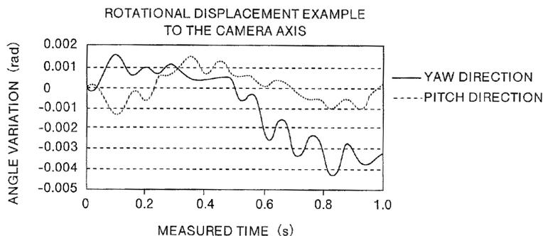
**Figure 4.** Angular camera displacement due to handshake<sup>10</sup>
