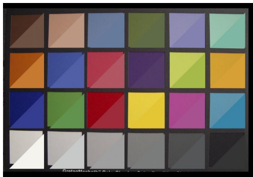
Figure 10: To visualize the color differences a file can be used which has the values of the original chart in the lower right corners and the value of the test image in the upper left. The Photoshop sample file can be downloaded from 14.
