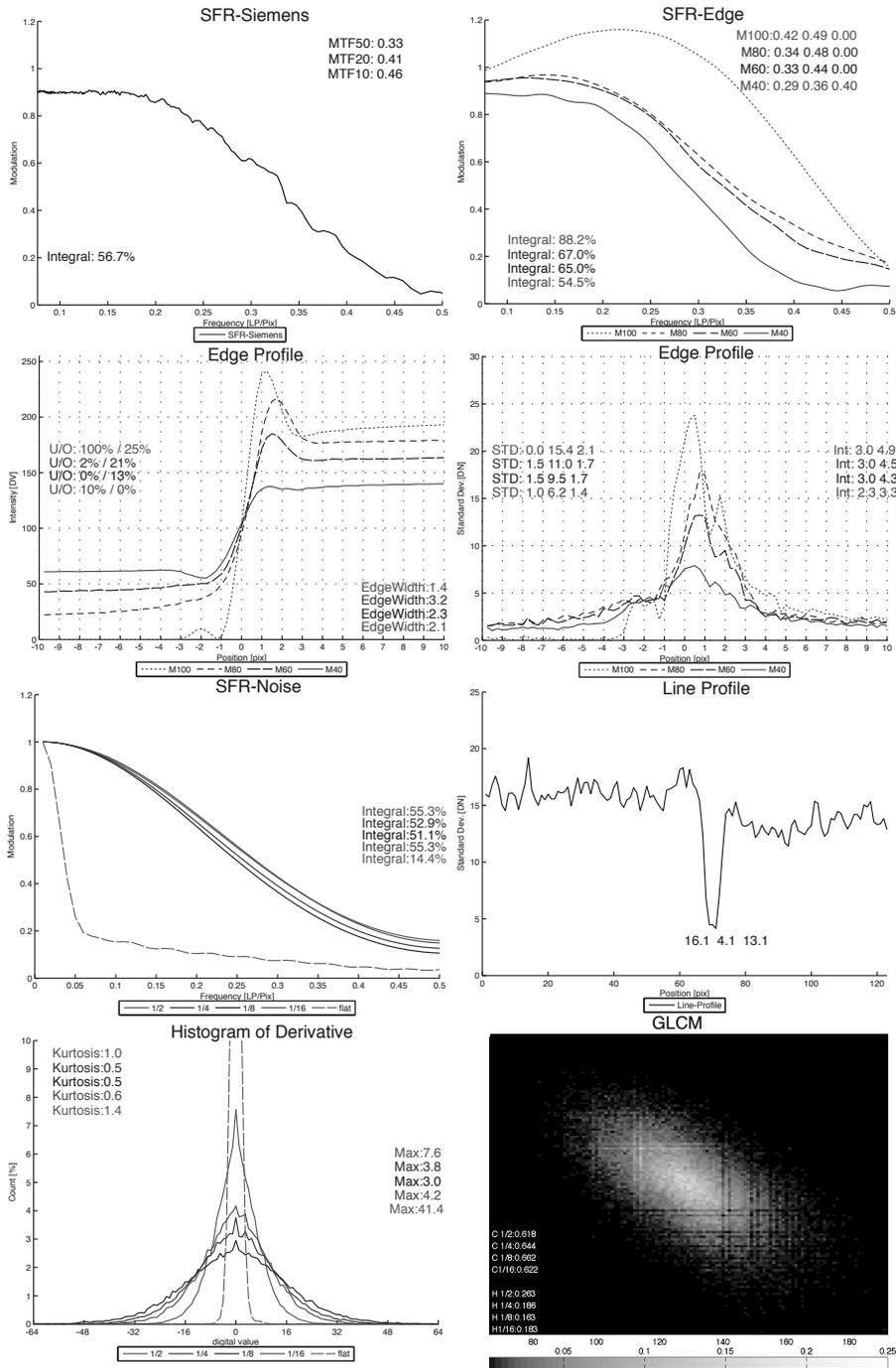
Figure 7. Graphical Results of a consumer compact camera (ISO100)
