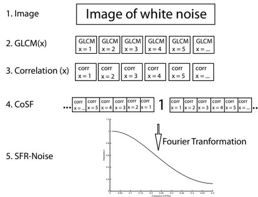
Figure 3. Calculating SFR-Noise
