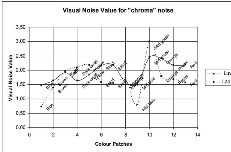
Graph 1: Reports the measured visual noise value for each colour patch,once for the visual noise value determined with the CIEL\*u\*v\* and once with the CIEL\*a\*b\* formula.
