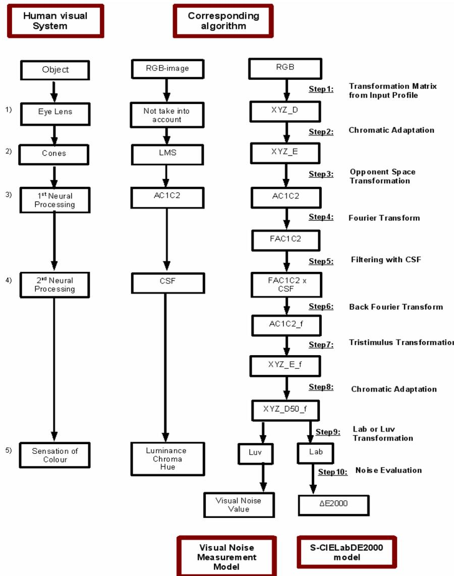
Fig 3 : Scheme of the implemented human visual algorithm<sup>2</sup>
