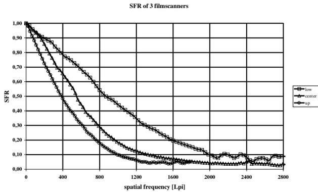
Figure 3. SFR results of three different film scanners
