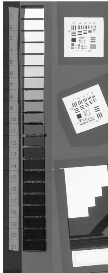
Figure 2. The test charts created by Image Engineering.
