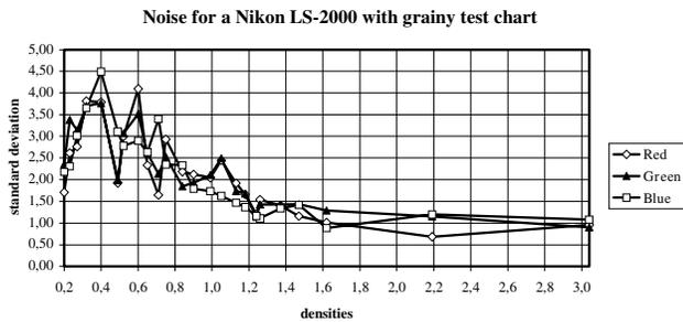
Figure 7. The measured absolute noise levels with a typical testchart using a Nikon film scanner.
