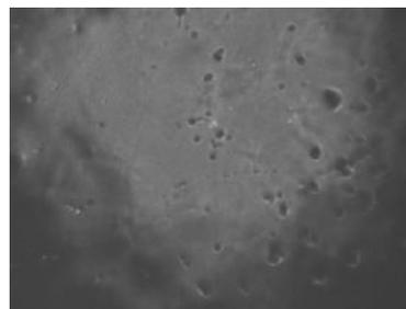
**Figure 6:** 50% magnification of a polymer coated paper
