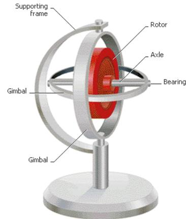
Figure 17: Mechanical Gyroscope [18]
