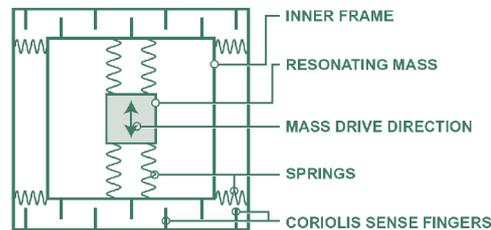
Figure 21: Schematic of the gyro's mechanical structure [21]
