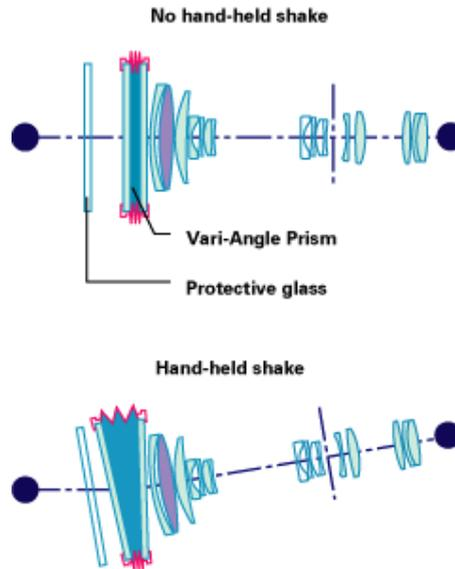
Figure 4: Vari-Angle Prism Image Stabilizer System [6]
