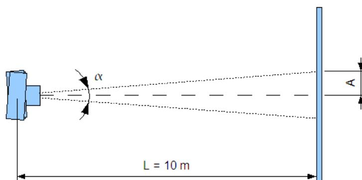
Figure 29: Measurement of the angular amplitude
