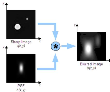
Figure 25: Convolution of a sharp image with a PSF
