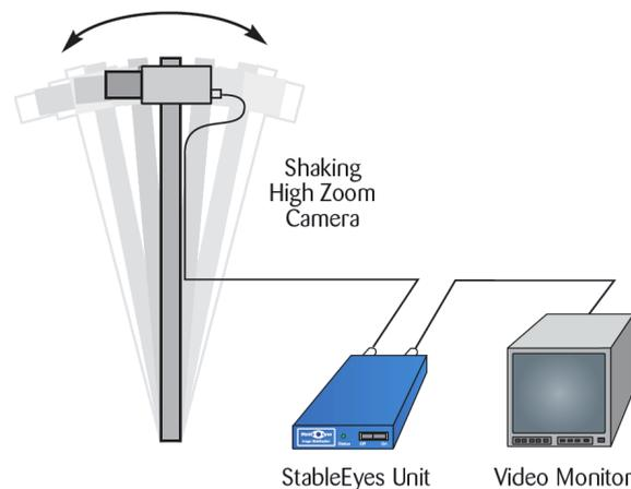
*Figure 13: External Electronic Image Stabilization [13]*
