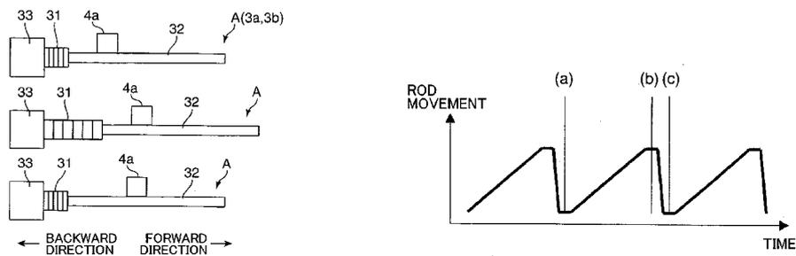
Figure 7: The principle of Minolta's piezo-actuator [10]
