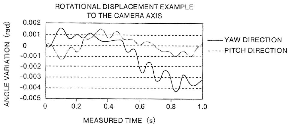
*Figure 31: Angular camera displacement due to handshake [11]*
