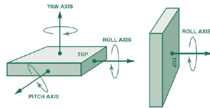
Figure 24: Mounting of a gyroscope [21]
