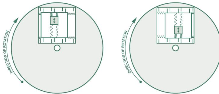
Figure 22: Gyroscopic precession [21]
