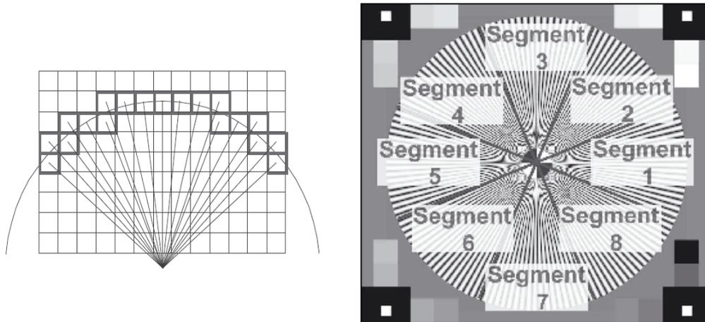
Figure 27: Pixel localization and averaging of segments[26]
