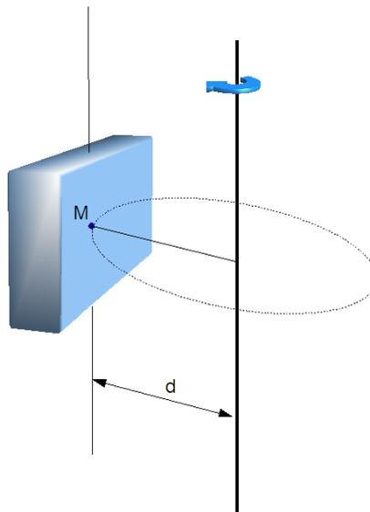
*Figure 33: Parallel axes theorem (according to [30])*
