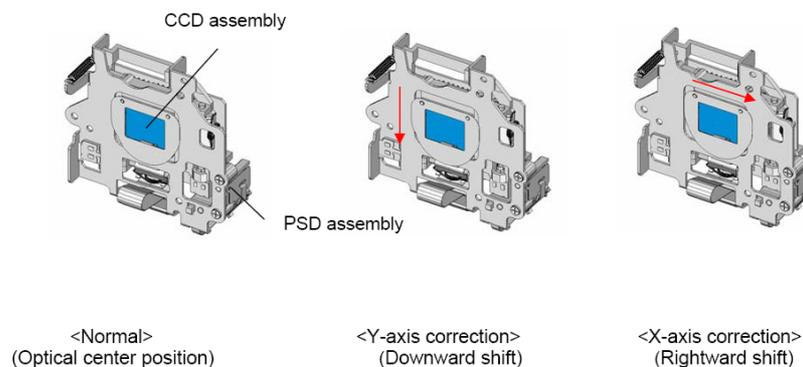
*Figure 8: Konica Minolta's CCD-Shifting mechanism [9]*
