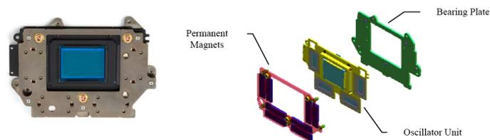
Figure 10: Shake Reduction unit by Pentax [12]
