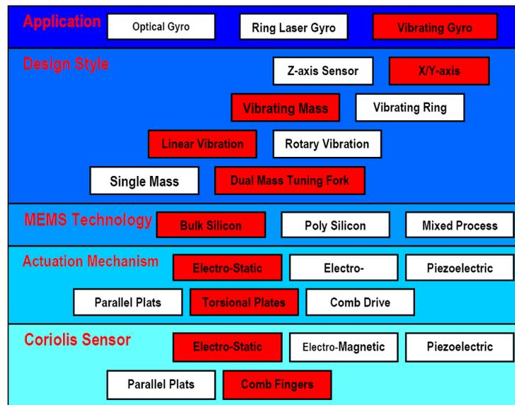
Figure 19: Variety of gyroscopic sensors [20]
