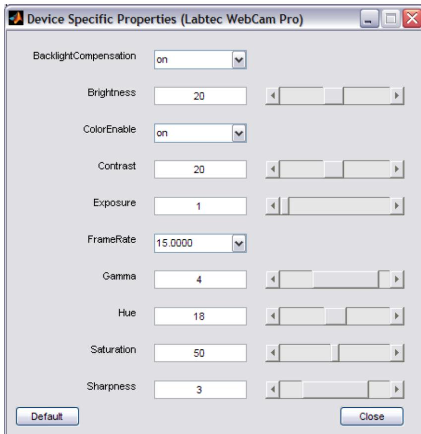
Figure B.3.: Device specific settings for Labtec WebCam Pro. The settings are dynamically collected from the adaptor DLL and summarized in the dialog window.
