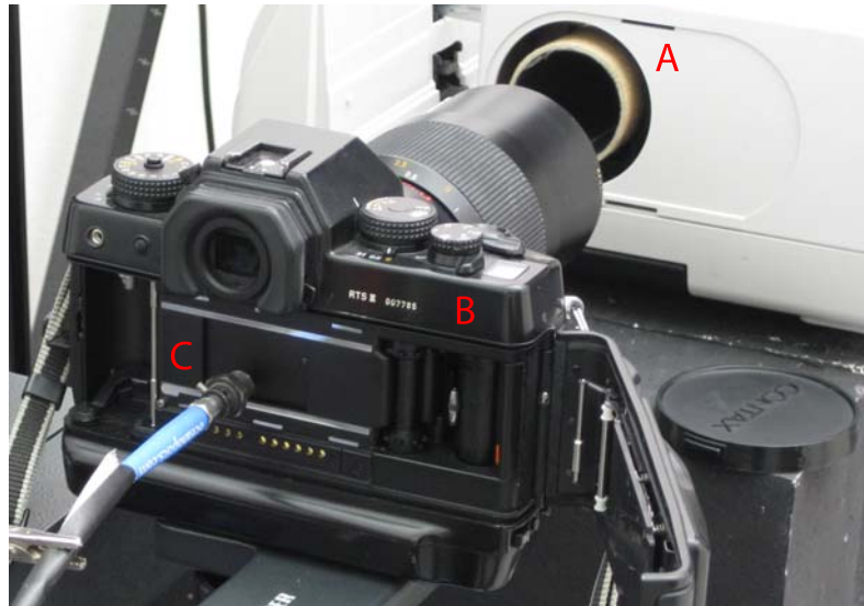
Figure 3.6: The used setup to evaluate the angle dependency of the interference filters. With A camSPECS, B 35 mm camera with open back, C spectrometer fiber-optics.
