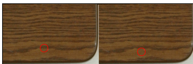
Figure 5.2: these two measuring points on the structured object result in a different luminance value
