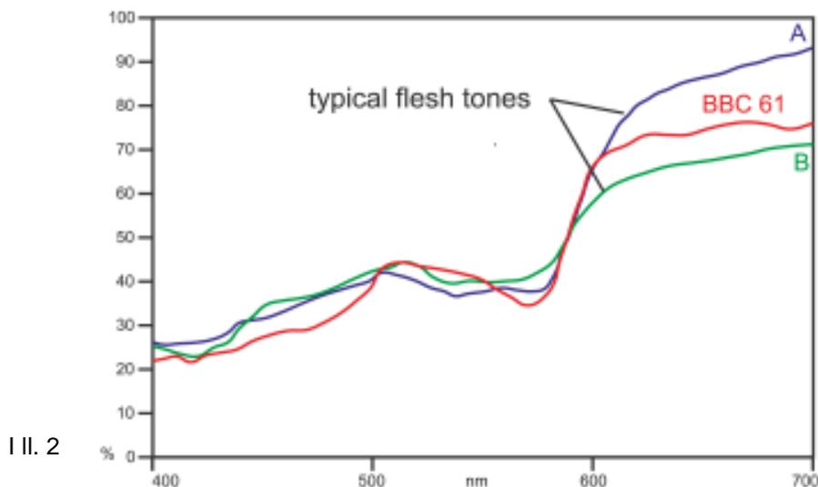
With this chart several color cameras can be adjusted simultaneously to an approximate uniform rendition of flesh tones. First cameras have to be adjusted with a logarithmic gray scale (TE108; TE109; TE153). By using the TE109 the change to be BBC61 can be made without changing f-stop. In combination with the T13 the chart is suited for testing flesh tone rendition of cine color films.
