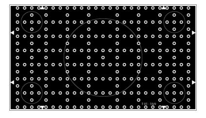
The test chart is designed to measure geometry of cameras and monitors.
