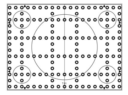
The test chart is designed to measure geometry of cameras and monitors.
