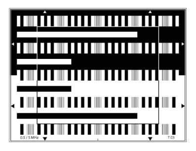
The T03 is designed for evaluating the uniformity of the modulation depth of TV cameras.
