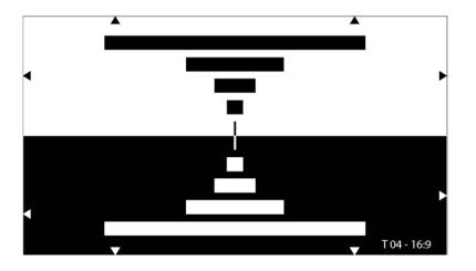
The bar test chart is designed for checking the transmission characteristics of TV cameras at intermediate and deep frequencies.
