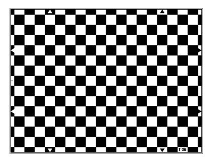
The T06 test chart is designed for checking geometry and resolution.
