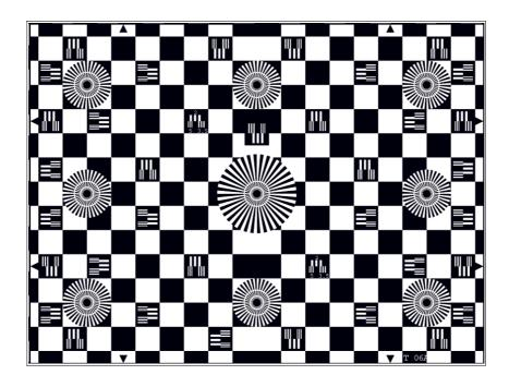
The T06A test chart is designed for checking geometry and resolution.
