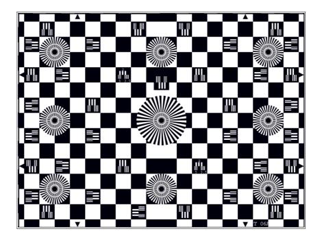
The T06A test chart is designed for checking geometry and resolution.
