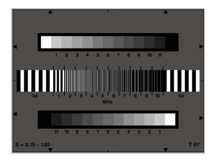
The test chart is designed for evaluation of the halftone reproduction and frequency response of the modulation depth of electronic cameras.
