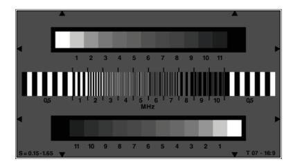
The test chart is designed for evaluation of the halftone reproduction and frequency response of the modulation depth of electronic cameras.
