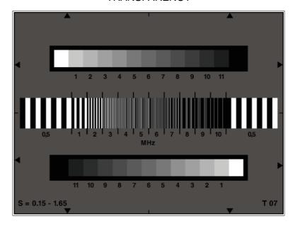
The test chart is designed for evaluation of the halftone reproduction and frequency response of the modulation depth of electronic cameras.
