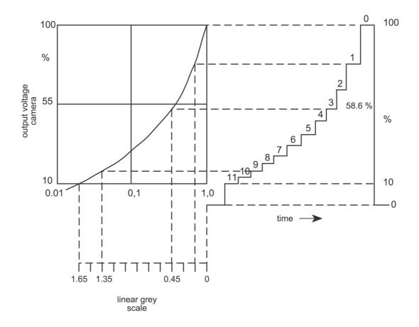
With the line rasters it is possible to determine the contrast transformation function. The reference value is the signal amplitude of the 0.5 MHz burst. To measure the CTF (contrast transfer function) not only in the middle but also on the upper and lower edges the camera has to be swiveled downwards and upwards. Care must be taken to avoid clipping of the signal to be measured at the black and white level.
