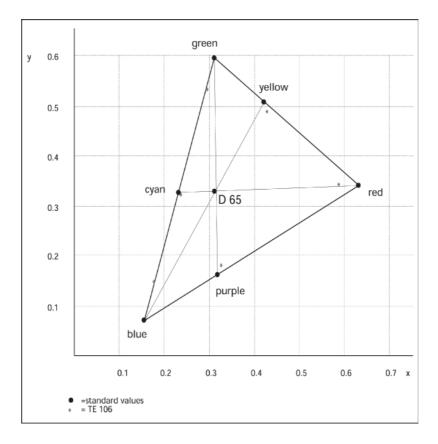
The brightness of the colors is matched with the electronic 100/75 color bar. To compare the luminance of the reflecting color with standard value, the following table shows the L\*-value in the CIE-L\*a\*b\*-diagram.
