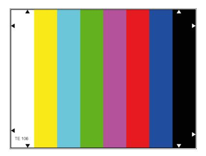
The test chart TE106 is designed for checking the color rendition of TV cameras.
