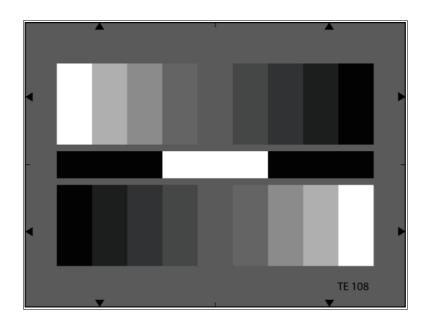
Two 9-graduated counter current gray scales are arranged on a gray background (D = 0.75), the gray scales being graduated logarithmically (gamma = 0.45). The output signal of an optimal gamma-corrected camera yields two 11-graduates counter current linear step signals. The contrast range of the gray scales is 50 : 1.
