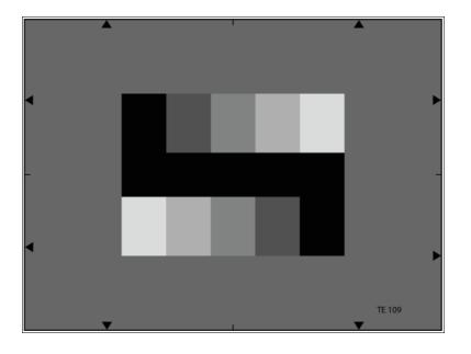
Two 5-graduated counter current gray scales are arranged on a gray background (D= 0.65), the gray scales being graduated logarithmically. Related to the densities of the gray scales: gamma = 0.45. Related to the transmission values (brightness): gamma = 2.2, that being exactly the reciprocal value of gamma = 0.45
