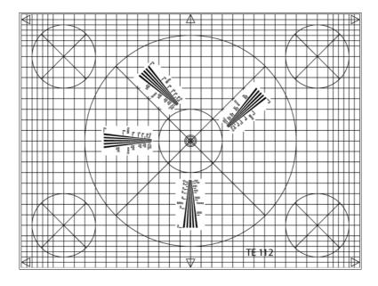
A grid structure consisting of 23 horizontal and 35 vertical lines is arranged on a white background. 3 grid lines each divide the outer 3 grid rows in the middle. The width of the grid lines is 0.15% of the picture width. The large circular line has a diameter of 83 1/3% of the picture height, the 5 small circular lines have a diameter of 25% of the picture height.
