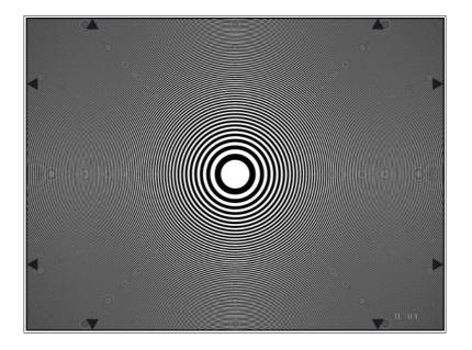
The zone plate test chart is designed for checking the resolution characteristics and "cross color" interferences of TV cameras and TV transmission systems. The test chart shows a zone plate over the whole image area where the spatial frequency of the rings has a linear increase towards the edges. In horizontal direction spatial frequency reaches 8 MHz and in vertical direction 6 MHz at the edges of the test chart. In the corners of the test chart spatial frequency is 10 MHz.
