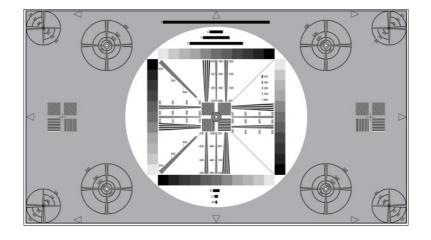
The TE117 is designed for quick (mainly visual) appraisal of transmission characteristics of HDTV cameras.
