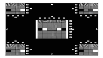
The TE118 is designed for checking the resolution characteristics of HDTV cameras. The frequencies to be resolved are indicated in cph (cycles per height).
