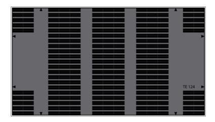
The test chart with an aspect ratio of 16:9 shows in the middle area 9 blocks containing 42 resolution patterns each. The corner fields have 20 resolution patterns.
