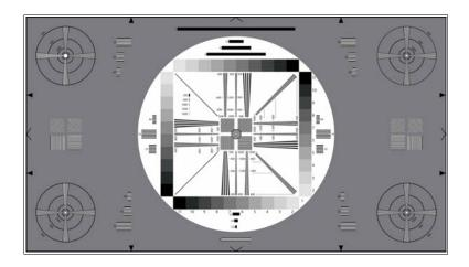
The TE128 is designed for measuring and quick (most visual) appraisal of transmission characteristics of high resolution non-broadcast cameras.
