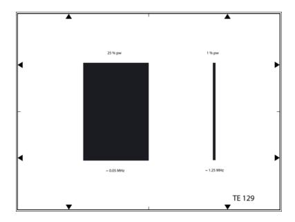
The test chart is used to measure low and intermediate frequency response (streaking) and flare in video systems.
