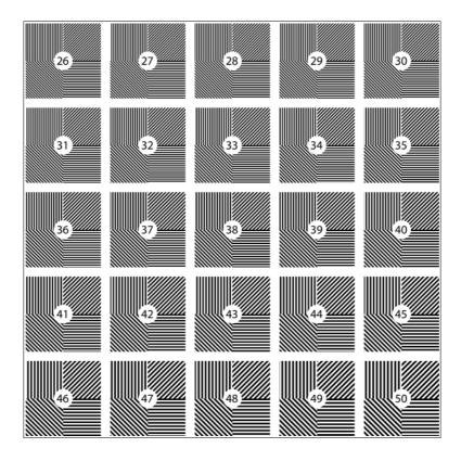
The chart is designed to do resolution measurements in a range of 2 - 0.5 linepairs per millimeter.
