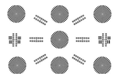
The test chart is used for evaluating the resolving power of a cine camera.
