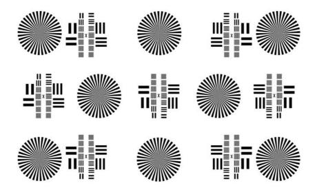
The test chart is used for evaluating the resolving power of a cine camera.
