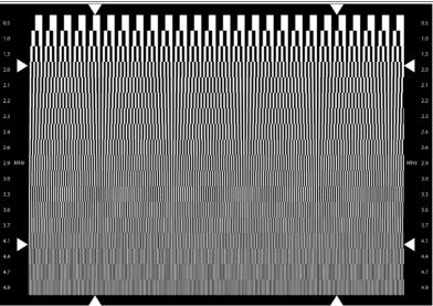
The TE144 was developed in a private German testing laboratory and serves particularly for evaluating the frequency response of consumer camcorders.
