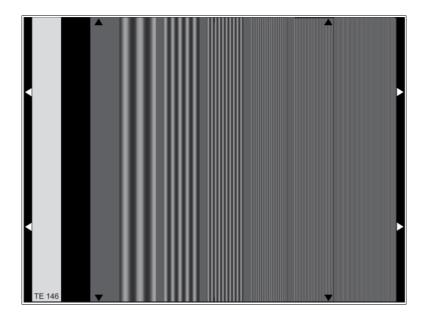
The TE146 reproduces the test signal, line 18, as specified in CCIR recommendation 473. With the aid of measuring instruments test signals can be evaluated in a simple, and partly automatic way.
