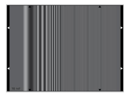
The TE147 reproduces the test signal, line 18, as specified in CCIR recommendation 473. With the aid of measuring instruments test signals can be evaluated in a simple, and partly automatic way.
