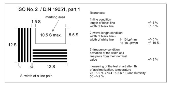
The ISO test pattern no. 2 consists of 26 groups of 2 x 5 line pairs which are arranged at right angle to each other. The line pairs have a nominal value of 1.0 to 18 lp/mm. The nominal value increases by factor 1.225 (  $\sqrt[6]{2}$  ) from one group to the other, i.e. the lp/mm value doubles after each 6 groups.
