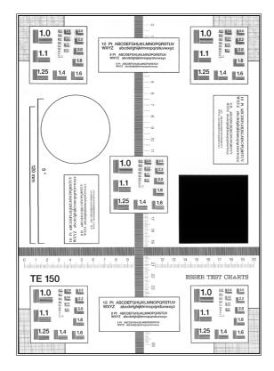
The test chart can be supplied as a foil or a reflectance chart, alternatively positive (see fig.) or negative. The foil is available in 0.10 or 0.18mm thickness. Image size is 297x210mm (DIN A4), external size is 303x216 + -1 mm.
